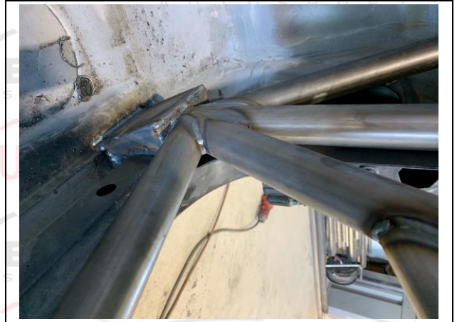
PHOTO 6 FRONT ROLLBAR TO FLOOR ATTACHMENT
