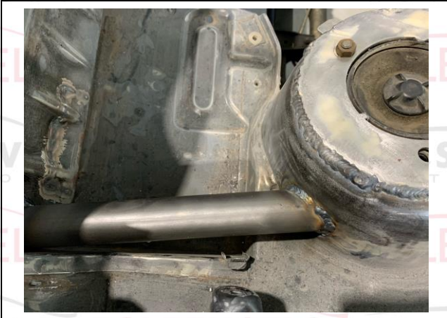
PHOTO 9 ATTACHMENT TO FRONT SUSPENSION
