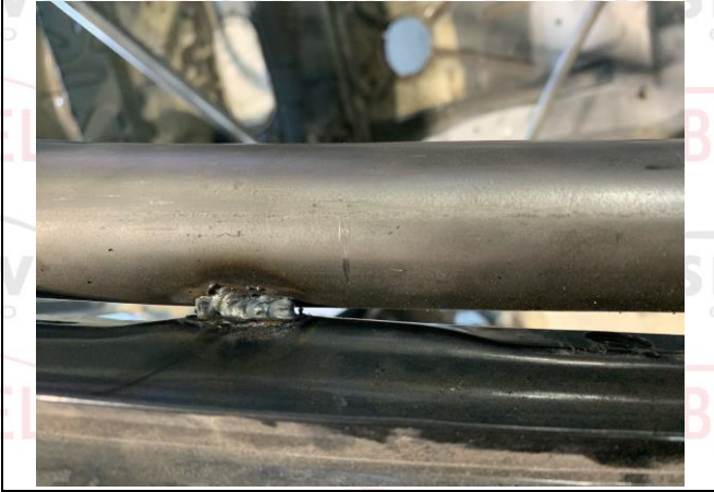
PHOTO 7 FRONT ROLLBAR TO "A" PILLAR ATTACHMENT
