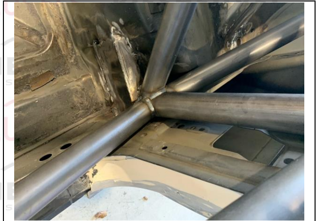
PHOTO 4 MAIN ROLLBAR TO FLOOR ATTACHMENT
